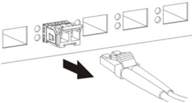
**Figure 20** Opening the Transceiver's Latch Example
