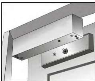
Demonstration of I Bracket Installation
