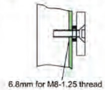
Inside: Drill a hole diameter is 8mm fold the plastic straight pin
