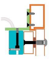
The power cable is exposed outside when installing the old type L bracket, it is not elegant and easy to be destroyed.
