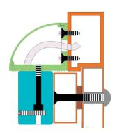
The power cable can be concealled inside the new type LC bracket, it is elegant and the cable can be protected
