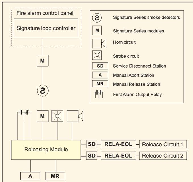
**Release Circuits 1 & 2** **Release Circuits.** The GSA-REL includes two supervised release circuits, each of which provides fire suppression control to different areas of a protected space. The releasing circuits actuate solenoids on the suppression agent tanks according to pre-defined release routines. These solenoids release the agent into the protected area. Both circuits operate together.
