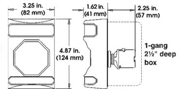
The service disconnect switch is used to temporarily disable the fire suppression system. One switch is installed on each of the two release circuits between the GSA-REL and the RELA-EOL end-of-line relay. Opening the Service Disconnect Switch allows the fire alarm system to be tested without activating the fire suppression system. The operation of this switch causes a trouble signal at the control panel.
