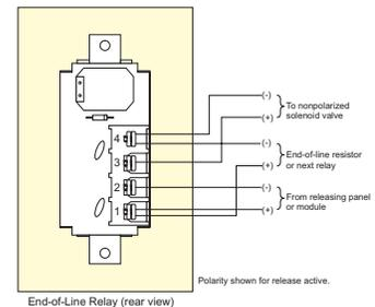
The End-of-Line Relay facilitates the connection of a non-polarized releasing solenoid to a supervised, polarized releasing circuit. One relay is required per release solenoid.
