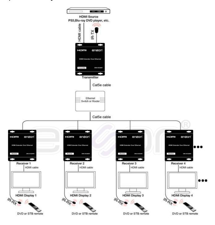
Note Connect HDMI Transmitter port and Receiver ports to the Ethernet Switch
