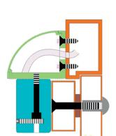
The power cable can be concealled inside the new type LC bracket, it is elegant and the cable can be protected
